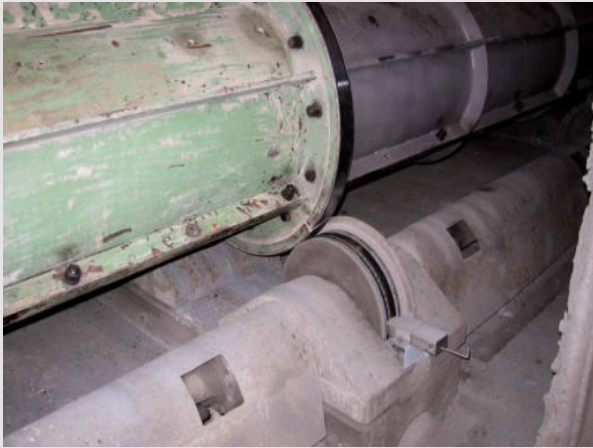
Friction drive asphalt drum
